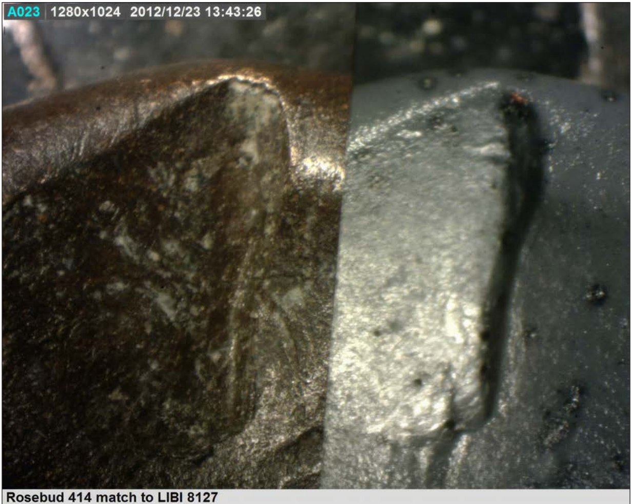
Figure 19. Microscopic image of Rosebud Spencer 414 fired in a Ball carbine compared to a cast of Little Bighorn Spencer 8127 also fired in a Ball carbine. Note the small scar near the top of the firing pin mark in both, which is one individual characteristic that aided in determining the two cases were fired in the same gun.
